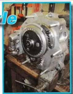
TOP, Gary Berg installs the gear cluster into a Rhino cased, Berg 5-Speed. ABOVE, this 5-speed assembly shows some of the new improvements Gary makes during current builds. Most of these upgrades are designed to allow more lubrication to access the main-shaft bearing.
