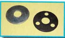
ABOVE, fifth gear stop washer is also modified on the right. Gary machines three large (.500-inch) holes into the face of this washer. BELOW, Berg drills three additional holes into the side of the billet mainshaft bearing retainer. These holes are placed between the four mounting holes already machined to the face.
