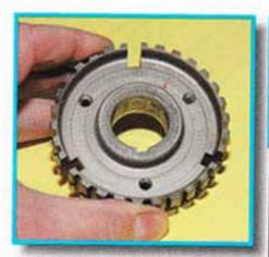
ABOVE, the fifth gear slider receives three new oiling holes, evenly placed between the dog slots. Hole size is 200-inch, then chamfered to allow more oil to pass through to the bearing.
