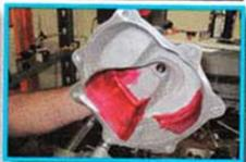
allow as much oil as possible to flow into the mainshaft bearing and 5th gear race/bearing.
